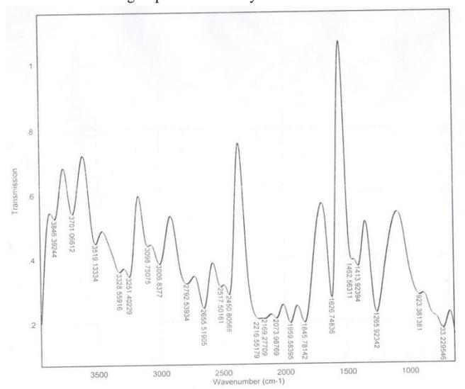
Figure 2: FTIR Spectra of Water Hyacinth
