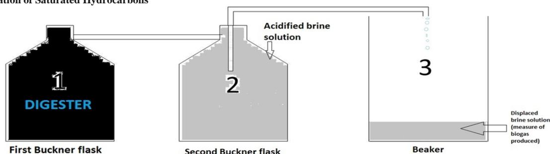
Figure 1: The experimental set – up for the biogas production
