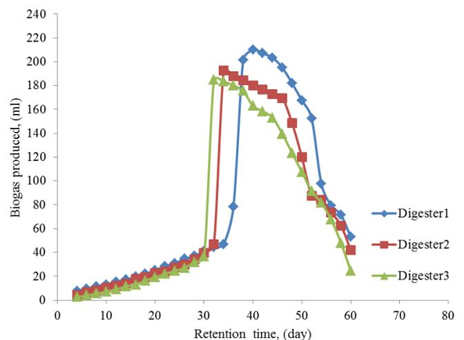
Figure 4: Biogas produced with retention time
